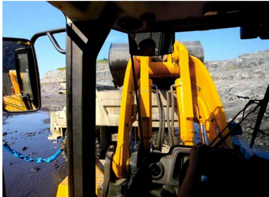
The cab protects the operator from noise and vibrations and is well ventilated. It has advanced climate control to handle the changing seasons and is completely sealed to prevent dust from entering the work place.
