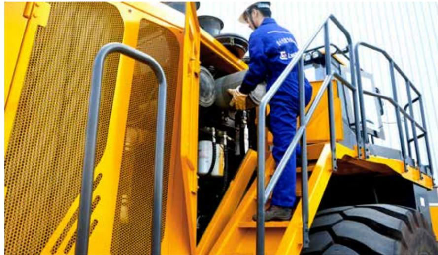
Maintenance speed and access is further improved with sturdy handrails, fitted as standard, which enable safe and easy access to the upper structure.
